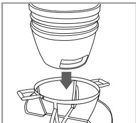
Take all parts out of the grill before lifting. With the help of a second person, lower the grill into the Stand by holding the back hinge and bottom of grill. As grill is lowered into stand, carefully switch out hands from bottom of grill to the ash drawer opening before reaching the outer ring of stand. Completely lower grill to bottom of stand.
