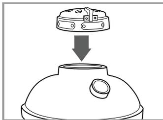
Close lid and press Top Vent onto top of Kamado. Be sure spring clips are fully engaged with calibrations facing the front of the grill.
