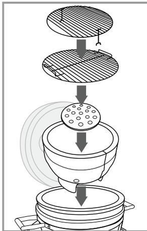
Lower fire bowl into the grill with the ash drawer opening facing the front of the grill. Place cast iron Charcoal Grate inside fire bowl. Place stainless steel cooking grate on top of the fire bowl.
