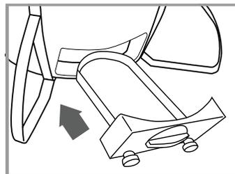
Slide Ash Drawer into ash drawer opening. When grill is cool, it is safe to remove ash from Ash Drawer. To remove Ash Drawer, use bottom knob on Ash Drawer, lift slightly and pull drawer out.
